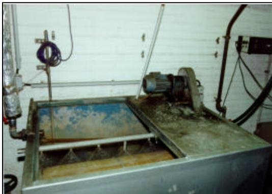
"The problem used to be that deposits started to build up after only a short operating time that it was impossible to remove" Mr. Sandor remembers. The expensive result was that the sieve had to be replaced frequently. Nowadays, the slurry is removed at intervals of four to five weeks with a high-pressure cleaning jet, and the sieve does not need to be replaced at all.
